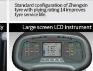
Standard configuration of combined Large screen LCD instrument overally handle integrating electro hydraulic reversing handle, steering and lights facilitates operation (hydrodynamic truck). monitor truck state. The instrument displays real time engine and truck fault information and humanized reminder.
