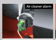
Standard configuration of air cleaner alarm reminds customer to maintain the air cleaner in time so as to protect engine and improve engine reliability.
