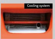
Enlarged aluminum plate fin radiator makes three kinds of temperature are controlled in a good range and effectively improves the reliability of the system.
