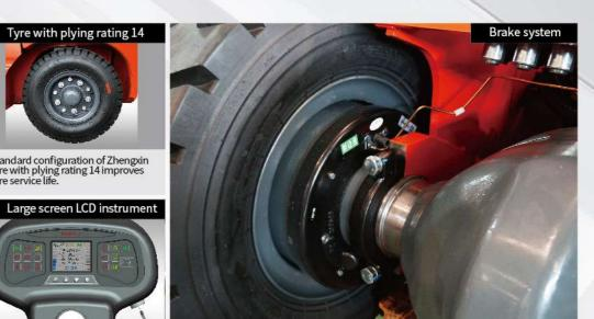
Upgraded brake drum and brake unit improves brake reliability and operation comfort.
