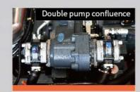
The application of double pump confluence hydraulic system provides oil supply as required and reduces energy consumption of the whole truck.
