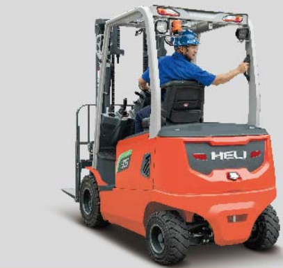
The rear handle and warning horn are designed for safer reversing operation.
