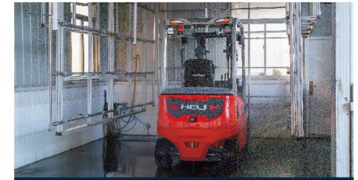
IPX4 waterproof: the vehicle is powered on to simulate a 15min short-time 5000L rainstorm test, and the vehicle can continue to run without failures.
