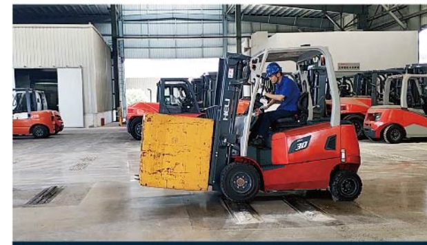
The truck passed simulation experiment of bumpy road.
